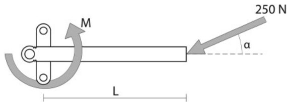
Figure 4: Forces and reaction moment in the sagittal plane in the standard bar.
