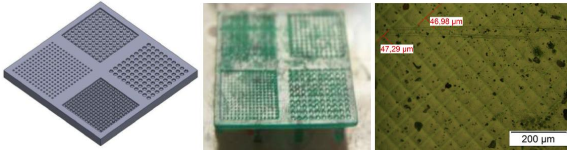
Figure 1. Micro features by DLP part (total part size 7x7x0.5 mm). Pixelation structure due to resolution of DLP. Courtesy University of Las Palmas de Gran Canaria.
