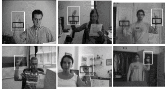
Fig. 3. Hand pose detection results showing wrists detections (dark rectangle) and complete hands (white rectangle).
