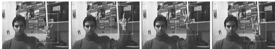
Fig. 5. Four frames (210, 220, 230, and 240) from a video sequence, where the centre of the tracked pattern is represented by a cross. The rectangle corresponds to the whole hand area computed through the use of hand-wrist proportions from the last wrist detected using the classifier.
