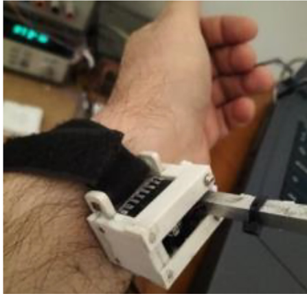
Fig. 5. Placement of the calorimeter on the volar area of the wrist.
