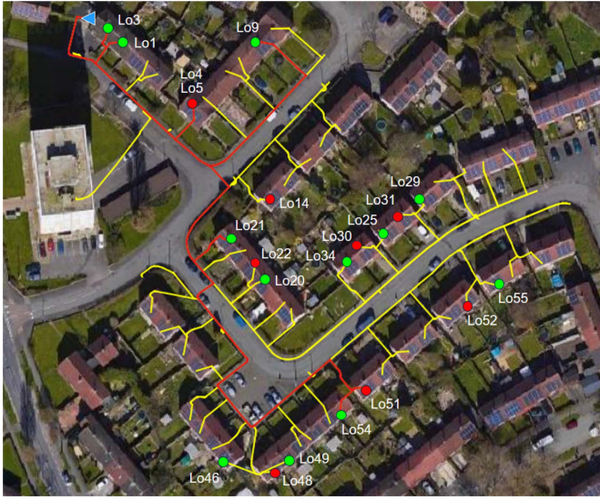
Fig. 8. Power flow tracing from pv51 in the modified IEEE European LV Test Feeder at 12:30 pm.
