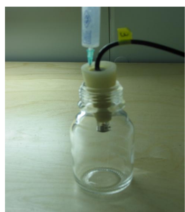
Fig. 2.- Incubation flasks showing the electrode and the pressure control
