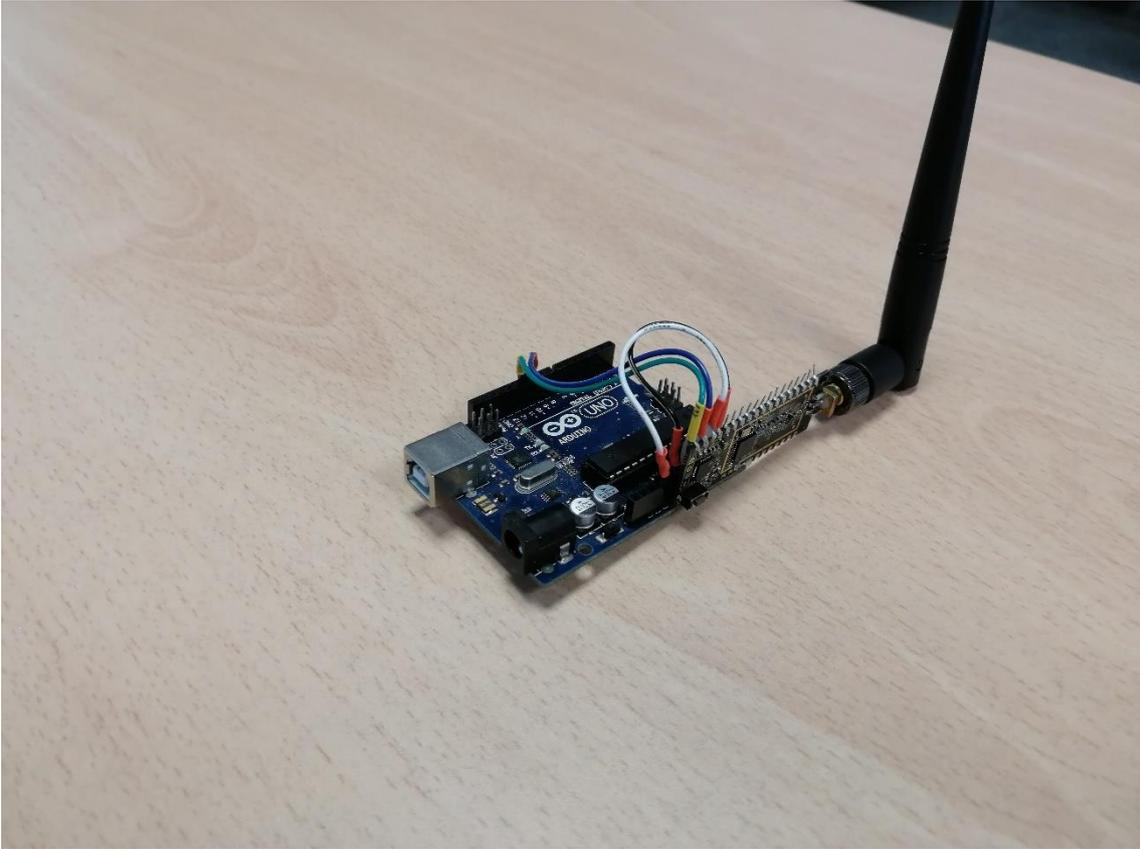
*Figura 42.Arduino Uno. Receptor LoRa.*
