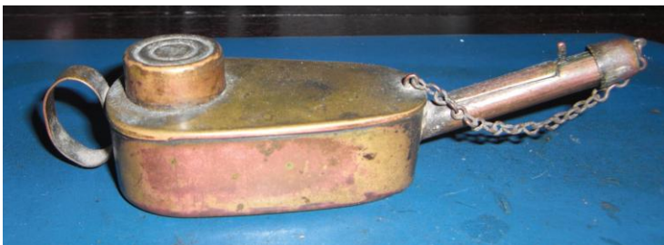
Detail of Aladdin's lamp, as it is called in the shop. Alcohol is introduced through an opening at the top and the size of the flame is regulated pulling the wick, which runs through the attached tube, in or out. The lamp is used to melt glue and detached pieces. Next to the lamp a glass bell used to cover the watches while you were working with them to avoid dust, 2009. Source: the author.
