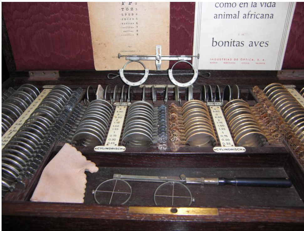
Detail of the wooden box that contains the lenses and frame used for eye testing, from manufacturer Nitsche & Günther, 2009. Source: the author.
