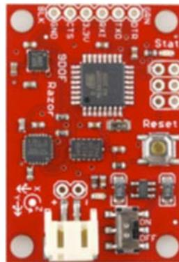
Figura 2.14. 9DOF Razor IMU
