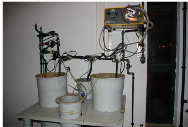
Figure 11: Automatic feeding system (stocking silos and pump)
