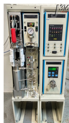
Fig 9: Pressurized liquid extraction method (own elaboration) Fig 10: PLE system (J316)
