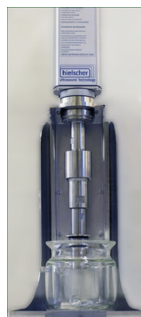
Fig 6: Ultrasound-assisted extractor (Petigny et al., 2013)
