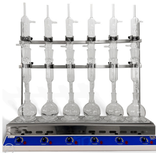
Fig 2: Soxhlet system (own elaboration). Fig 3: Soxhlet extractors (Kasalab S.A.S)
