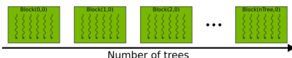
Figure 2: Bootstrap one-dimensional grid layout of the bootstrap kernel for nTree number of trees.
