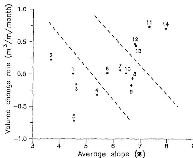
Figure 6.- Average volume change rate vs. mean foreshore slope for each profile. Numbers correspond to profiles.
