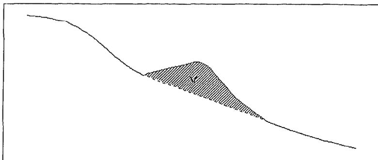
Figure 5.- Representation of the method followed to compute the volume of the subaerial sand bars (V).
