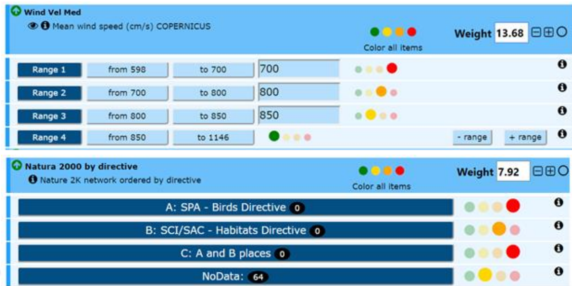
Figure 3 – Use case of parameter values divided into ranges (for numerical values e.g wind speed <7 m/s, 7-8.5 m/s , >8.5 m/s) and case of parameter values divided into categories (e.g. classification of Natura 2000 network)
