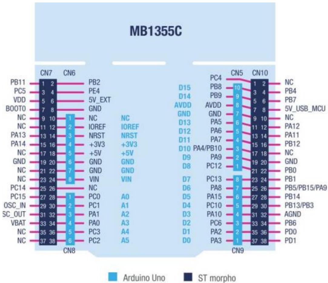
Figura 83. Pinout STM32WB55.
