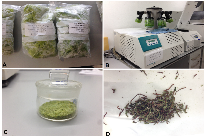
Figure 6. Frozen algae samples (A), lyophilizer, equipped with algae samples (B), grinded algae powder from Ulva rigida (C), lyophilized Hydropuntia cornea (D). (Photos: Jesse Theilen).
