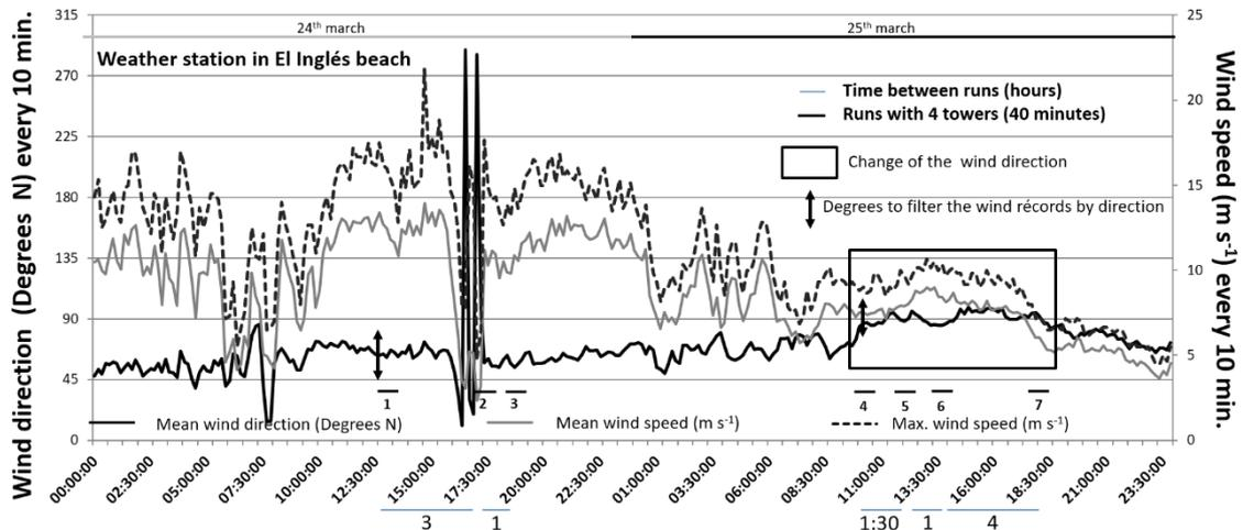
Figure 3. Wind conditions at El Ingles beach weather station (Kiosk 8). The graph shows the entire data set (every 10 min) recorded at the beach station during the experiment, the simultaneous wind sampling with 4 towers (Runs 1–7), and the change of wind direction between both days (black square).
