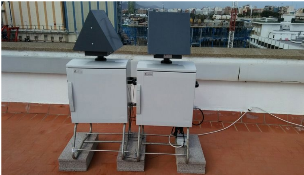
Fig. 3. High volume dust collectors (MCV brand) located on a building roof from Las Palmas de Gran Canaria Port authorities. Source: http://tecnobioambiental.ulpgc.es/2018/02/instalacion-de-captadores-de-alto-volumen-en-autoridad-portuaria-de-las-palmas/
