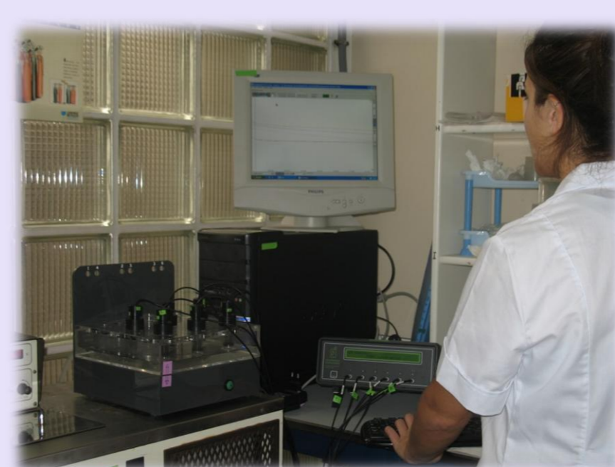
Figure 3. Temperature controlled incubation system. A 6-channel oxygen sensor was used to record changes in the dissolved O_2 concentration during the experiment.
