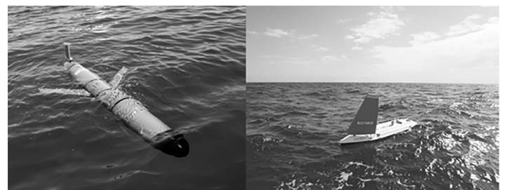
Fig. 1. The unmanned ocean vehicles described: Slocum G2 (left) and Sailbuoy (right)
