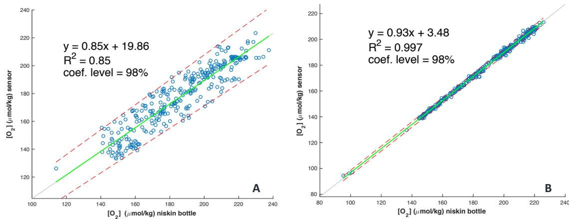
Figure 3. Comparison of dissolved oxygen concentration data of niskin bottles versus continuous data provided by the SBE43 dissolved oxygen sensor for Leg3 (A) and Leg5 (B) oceanographic cruises. Straight green line refers to the regression line. Red discontinuous line shows the confidence level for each oceanographic cruises at 98%. In both graphs the respective regression line equation and  $R^2$  is shown.
