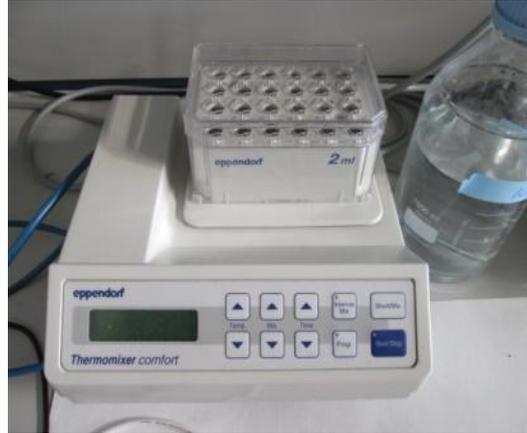
**Figure 5:** The thermomixer for incubation reaction.
