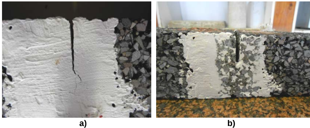
Prismatic sample of AC-VTL 11B PMB 25/55-65 with metallic filler (SPC<0.063 mm) and height 80 mm: a) Net initial crack depth of 19±1 mm, excluding the notch; b) Aspect of the same crack, completely closed in its entire depth, after an exposure time to microwaves of 110 s (starting temperature 20 °C).
