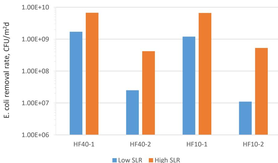
**Figure 3.** Average surface loading removal rates (g/m<sup>2</sup>d) of COD, NH<sub>4</sub><sup>+</sup>-N, DRP, and *E. coli* (CFU/m<sup>2</sup>d) in the first stage (HF40-1 and HF10-1) and second stage (HF40-2 and HF10-2) of the HF CWs for the periods of low and high SLR.
