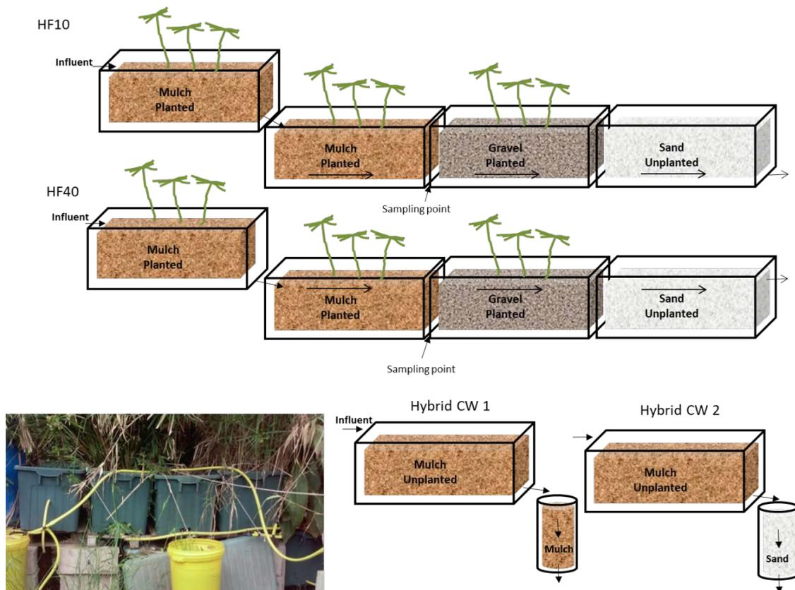
**Figure 1.** Scheme of the constructed wetland (CW) mesocosms employed in the study: multistage horizontal subsurface flow CWs (HF CWs) with water heights of 10 cm (HF10) and 40 cm (HF40); hybrid CWs with mulch-based HF CW followed by vertical subsurface flow (VF) with mulch (Hybrid CW 1) and sand (Hybrid CW 2). The photograph shows the hybrid CWs and the first unit of the multistage HF CWs.
