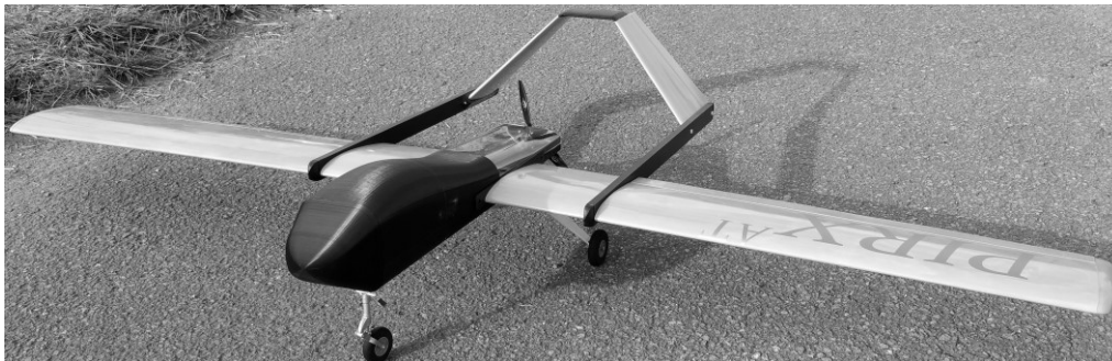
Fig. 1. Prototype of the UAV version with partially 3D printed airframes.
