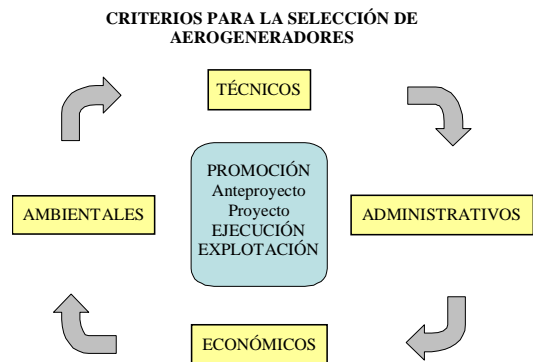
Fig. 3. Criteria to design a wind farm.
