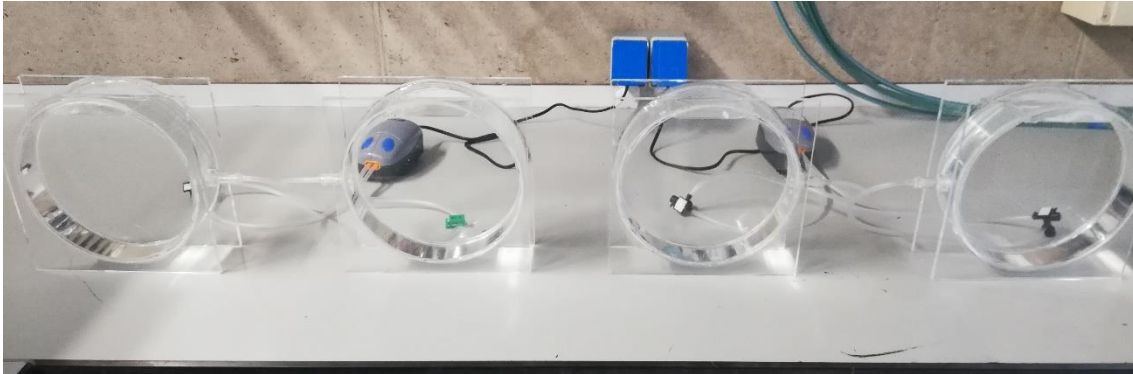
Fig. 4. Plankton kreisel used in microplastic ingestion experiments.
