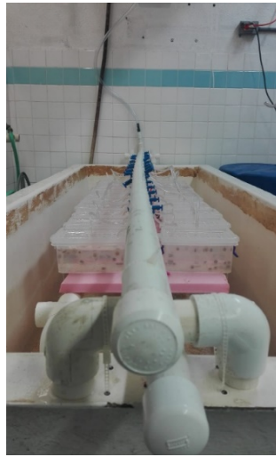
Figure 6. The containers where the sea urchins were maintained during the experiment. Each container had associated one flow of sea water and air.
