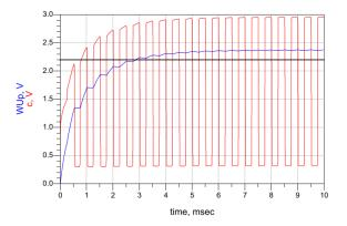
Figure 5. Preamble detector's input (signal 'c') and output (signal 'WUp').
