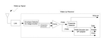
Figure 2. Low Noise Amplifier and Wake-up Receiver Overview.
