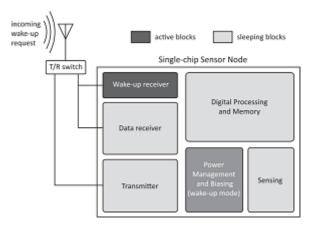
Figure 1. Block diagram of sensor node.
