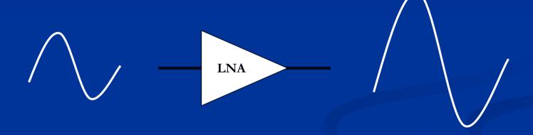
$$G = rac{V_{salida}}{V_{entrada}}$$
