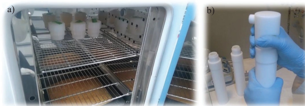
Figure 5.- a) Three aliquots in Savillex vessel (24, 48, and 72 hours at 90 °C and b) sample in microwave vessels.
