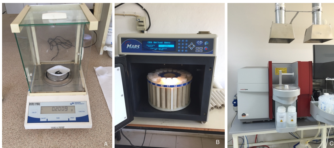
Figure 12 A) Weighing grinding of the dried algae B) Samples were treated in Microwave C) Atomic Absorption Spectrophotometer ContraAA with the part of graphite tube atomizer
