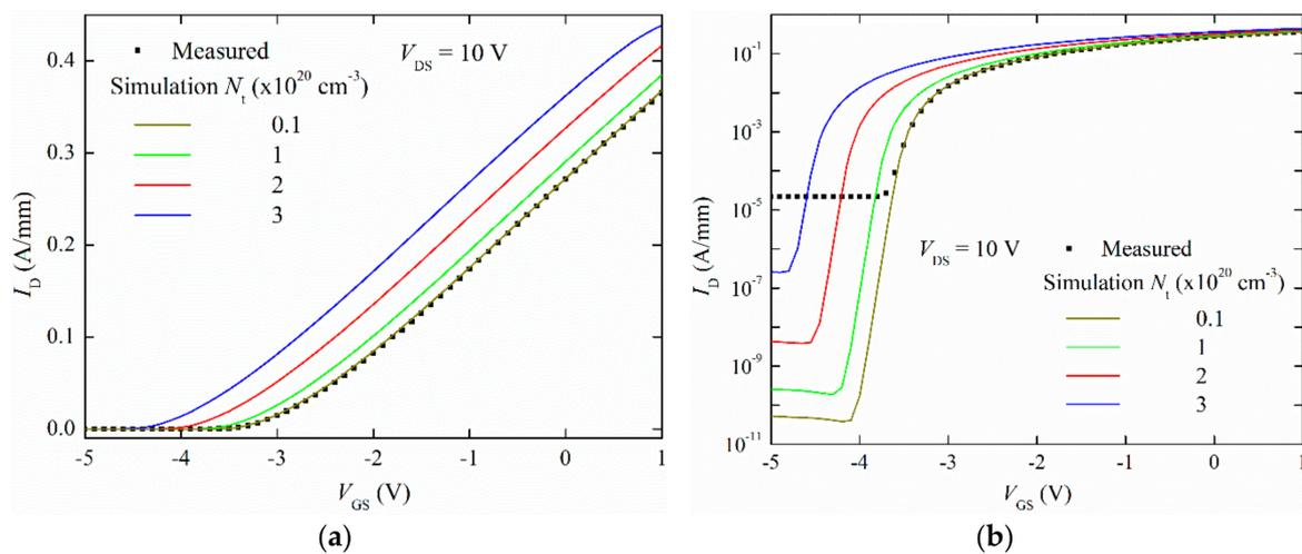
**Figure 2.** Measured (symbols) and simulated (lines) transfer characteristics for the AlGa<sub>N</sub>/GaN HEMT, for different traps concentration, with drain current in (a) linear scale and (b) logarithmic scale;  $V_{DS} = 10 \text{ V}$ .
