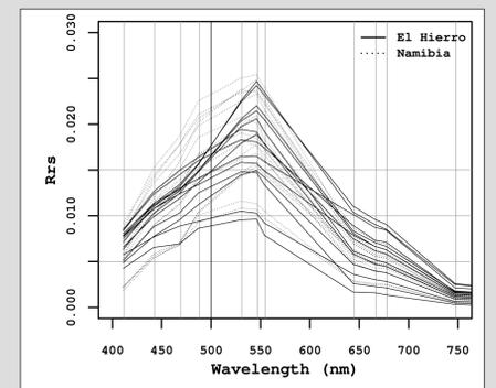
Fig.8.- Spectra of remote sensing reflectance of sulphide events off the Namibian coast and the El Hierro eruption.
