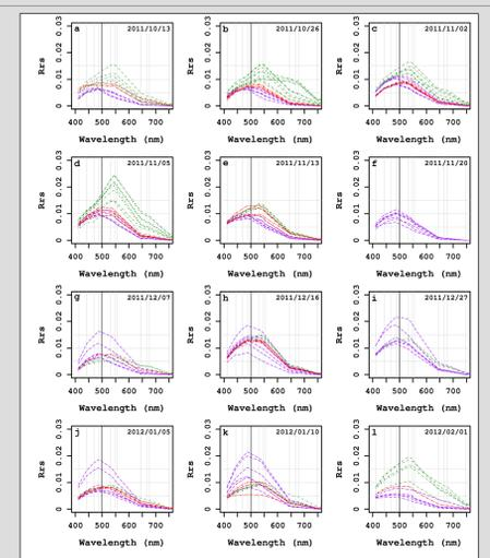
Fig.6.- Spectral of remote sensing reflectance showing variability over the volcanic plume on several dates. Green curves: Kd490 ≥ 0.15; red curves: 0.13 ≤ Kd490 < 0.15; purple curves: Kd490 < 0.13.
