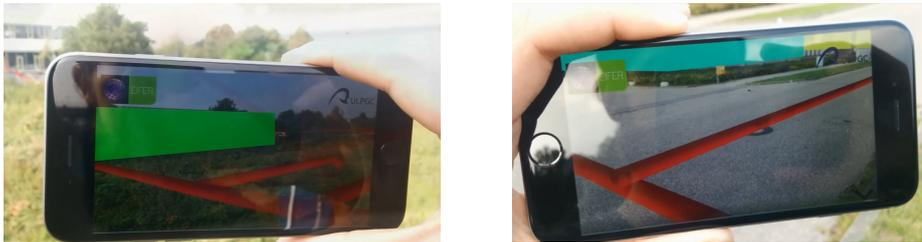
Figure 2, Underground infrastructure stored as CityGML visualised as AR on-site.
