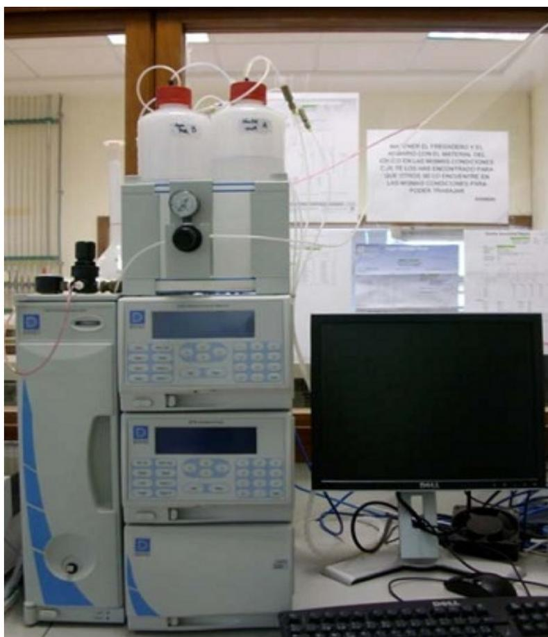
**Figure III.18: Ion chromatography equipment**
