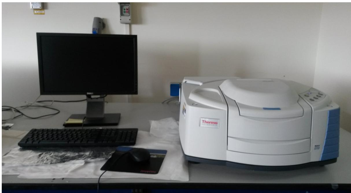
**Figure III.12 : Fourier transform infrared spectrometer model Thermo-Scientific-Nicolet iS10**
