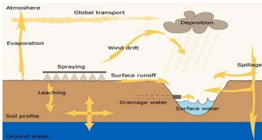
**Figure I.13 : Process showing the fate of pesticides in the environment [144]**
