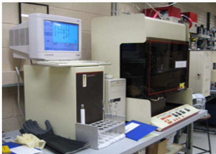
**Figure III.8 : BET Micromeritics 2010 instrument**
