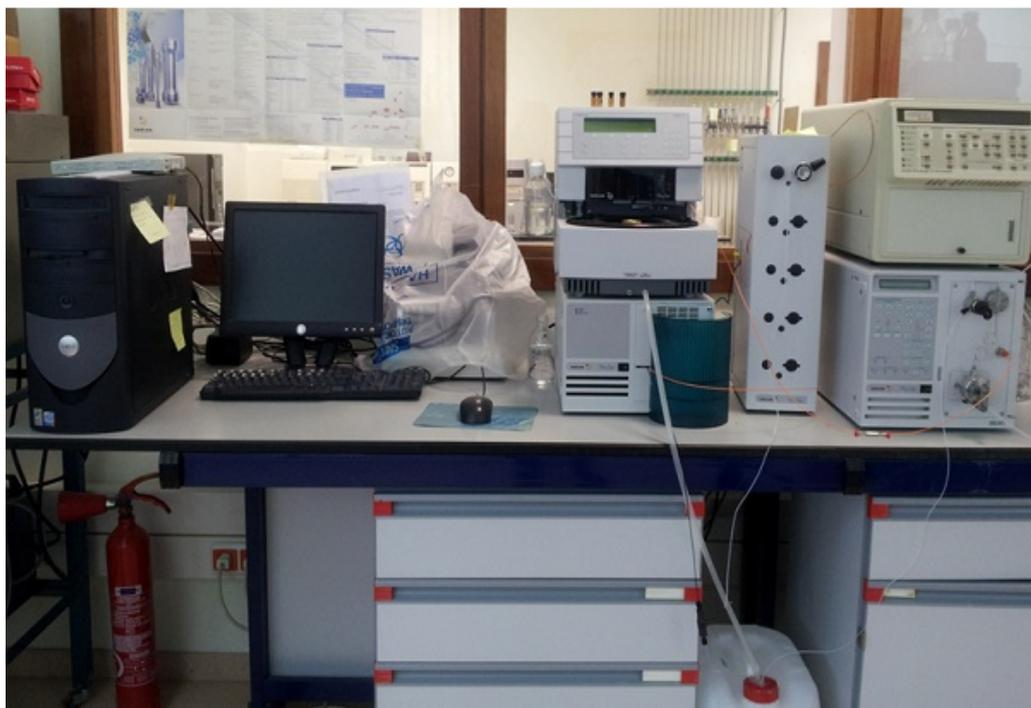
**Figure III.17: The second HPLC device**
