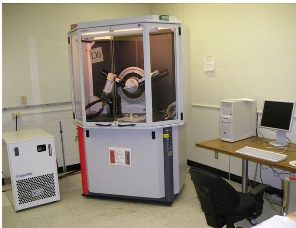
**Figure III.7 : Diffractometer XRD Bruker D8 Advance**
