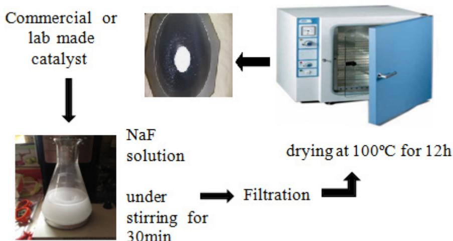
**Figure III.3 : The experimental process of doping the catalysts by fluorine (F-MO<sub>x</sub>)**
