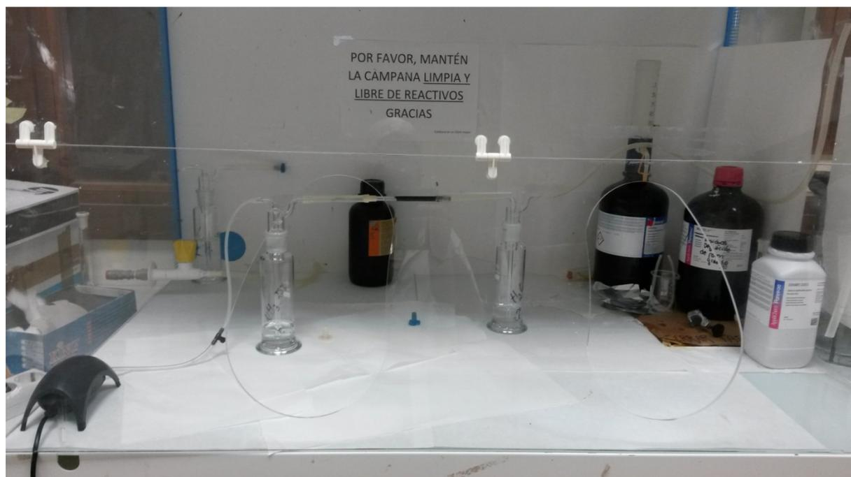
**Figure III.20: Experimental setup of gas phase studies**
