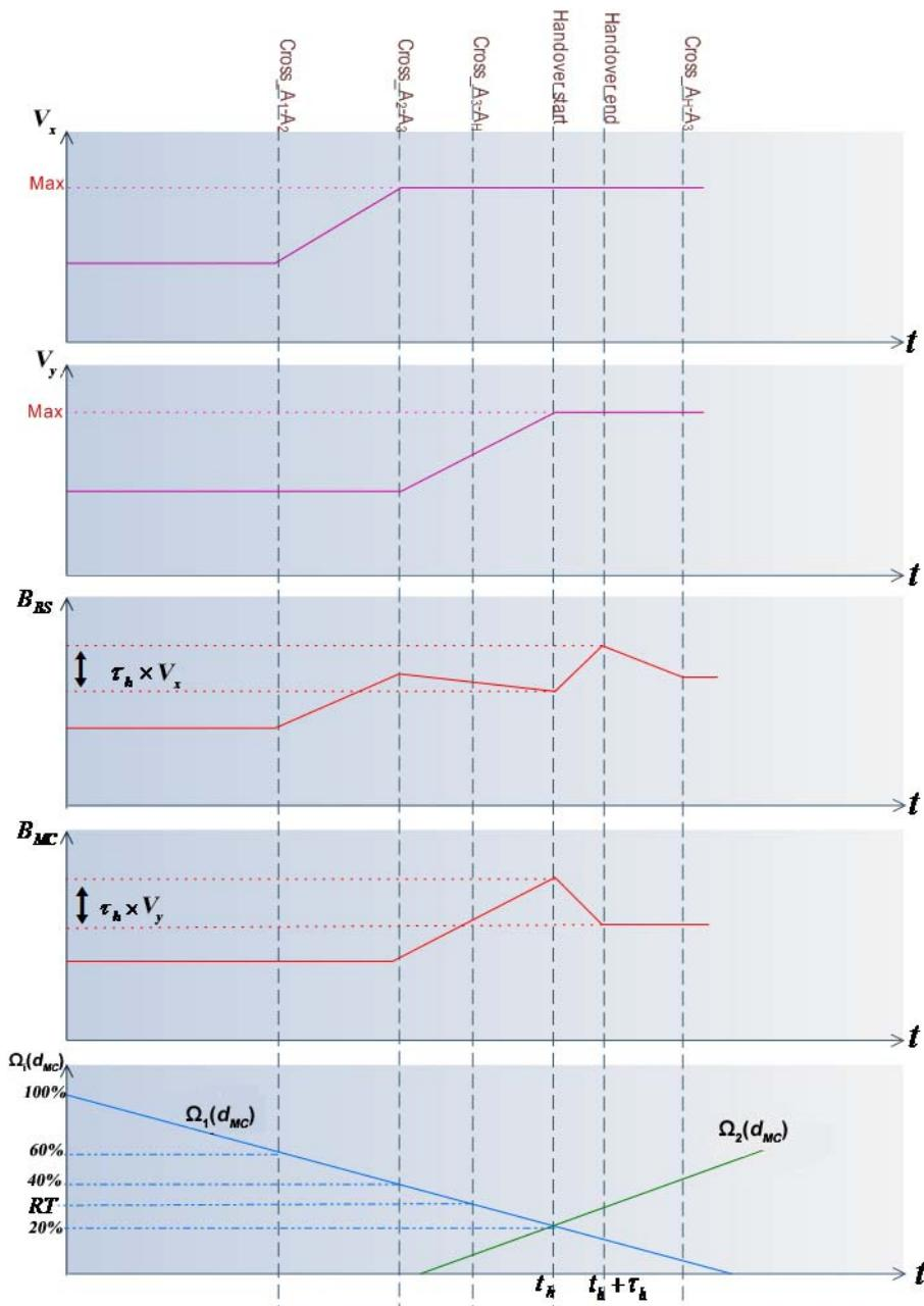
Figure 4.11: Impact of transitions actions on transmission speed and buffered video
