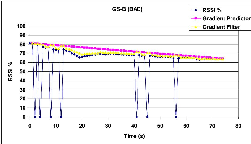
Figure 3.23: Gradient Filter test on RSSI measured values in the direction GS-B (BAC)
