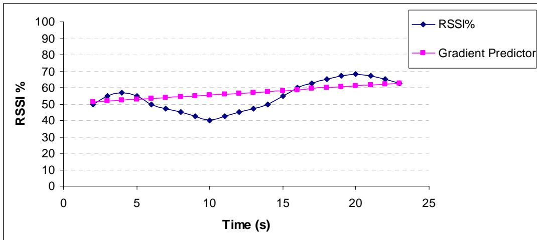
Figure 3.4: Prediction result of synthetic values when MC moves as shape F
