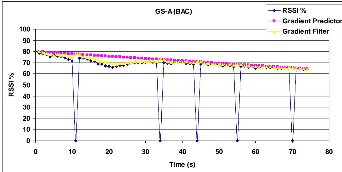
Figure 3.22: Gradient Filter test on RSSI measured values in the direction GS-A (BAC)
