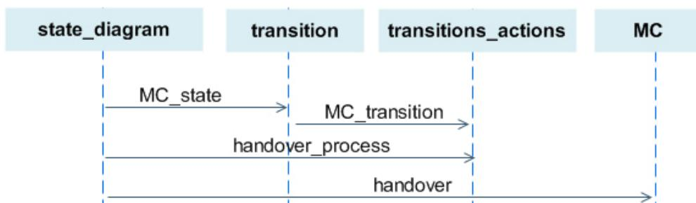
Figure 4.5: Signals generated by *state\_diagram* in case of handover
