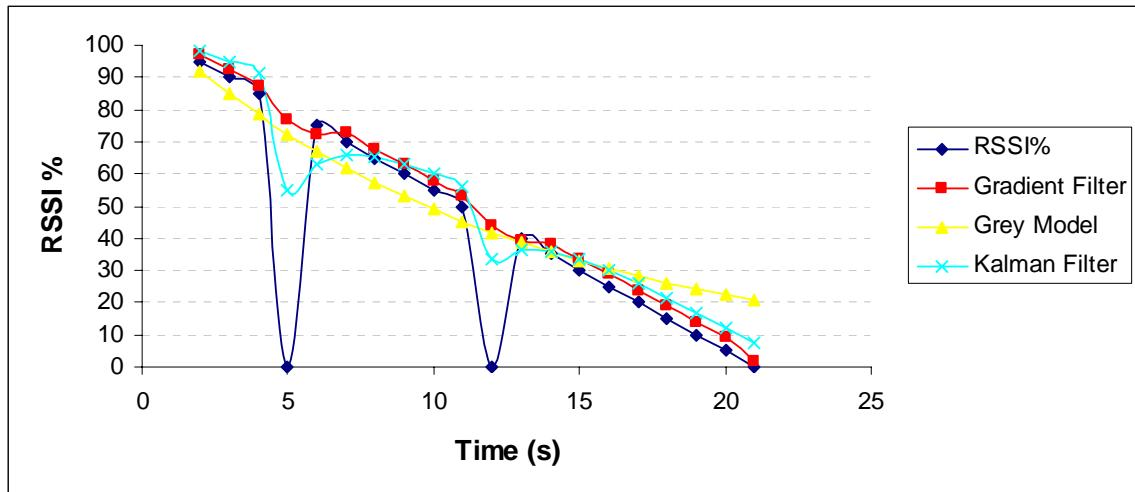
Figure 3.7: Filters results on synthetic RSSI values of shape A
