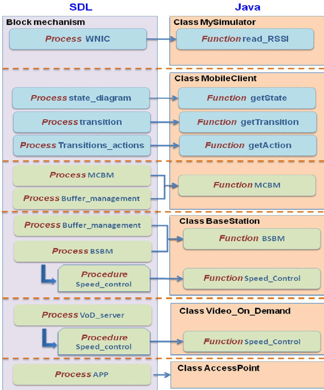
Figure 5.1: Derivation of the simulator from the SDL diagram
