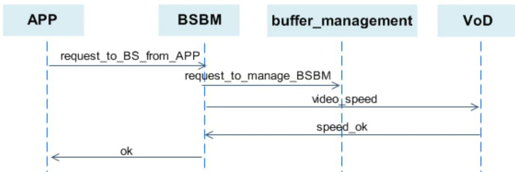
Figure 4.9: Signals exchange to control video transmission speed
