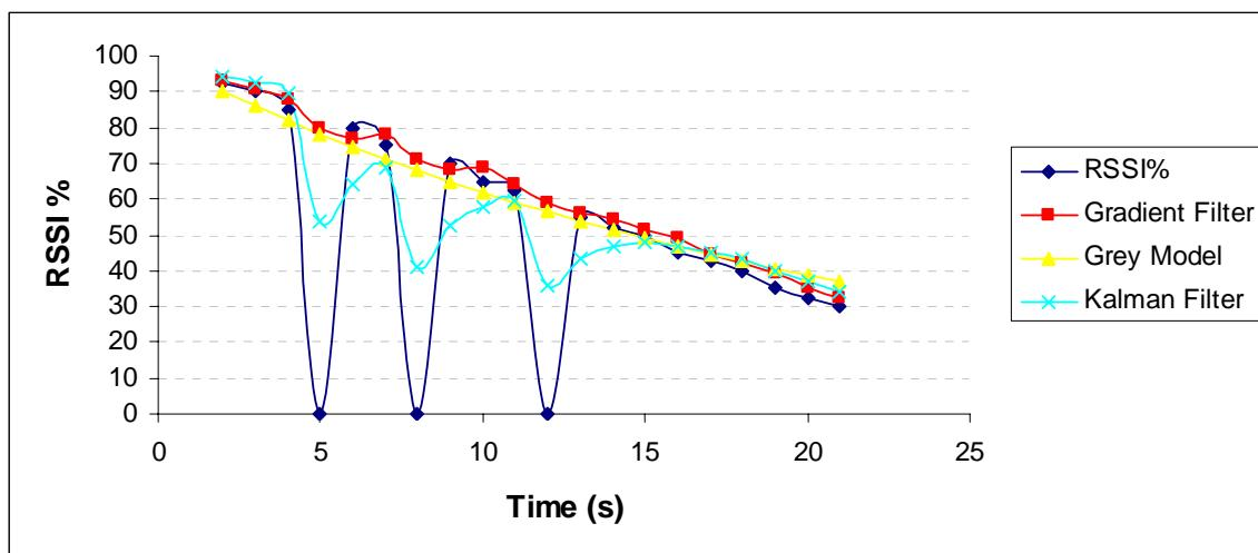
Figure 3.11: Filters results on synthetic RSSI values of shape E
