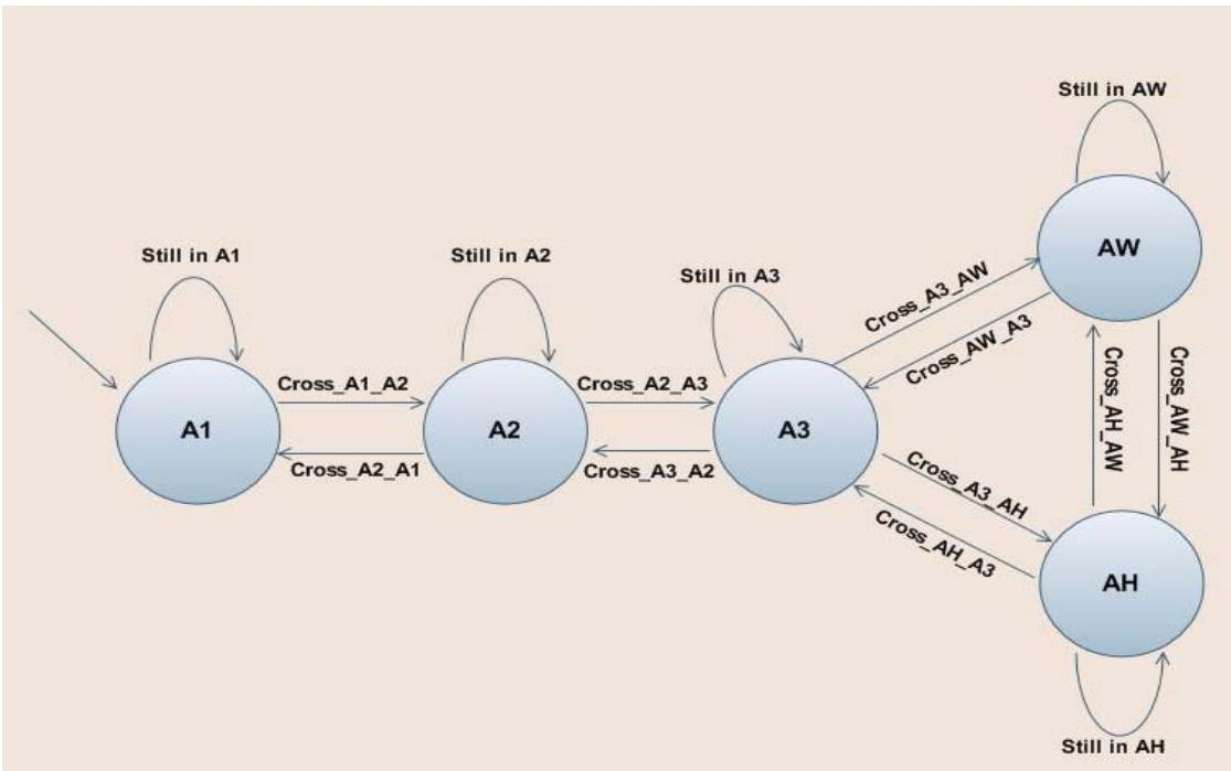
Figure 4.3: State diagram for MC transitions
