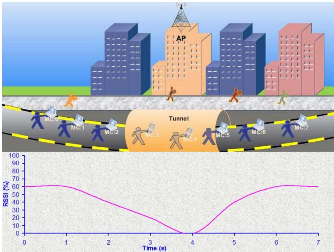
**Figure 1.4: The hole in case of MC passing through a tunnel**
