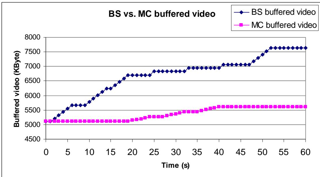
Figure 4.19: MC vs. BS buffered video of case 5
