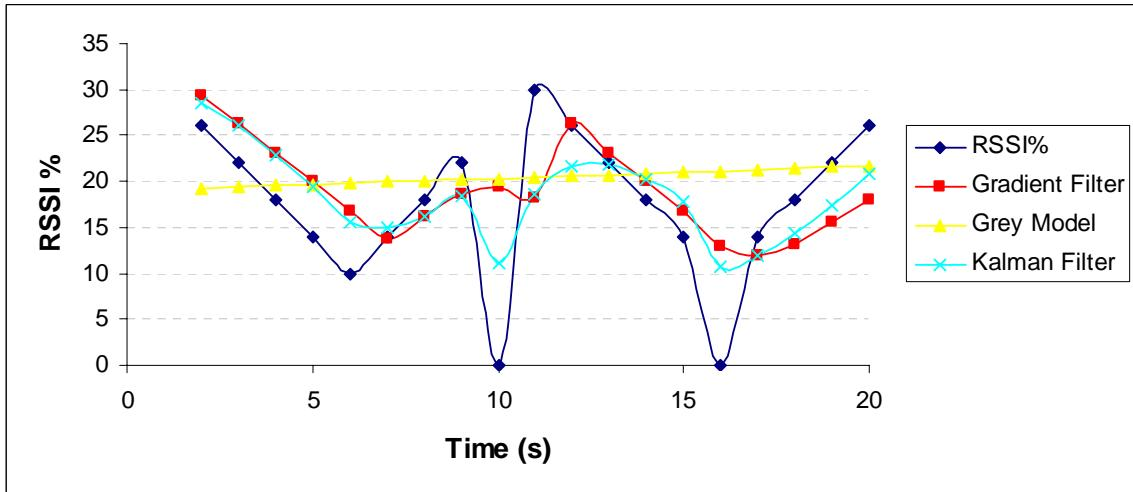
Figure 3.10: Filters results on synthetic RSSI values of shape D
