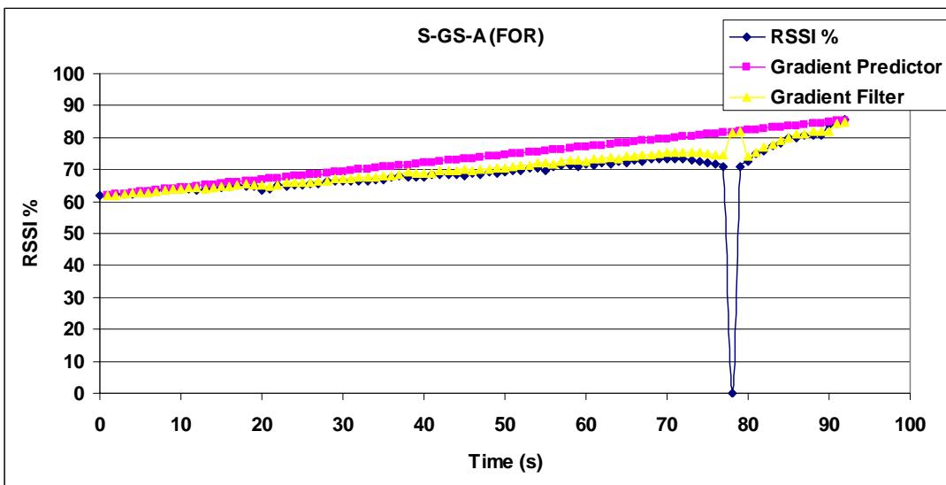
Figure 3.25: Gradient Filter test on RSSI measured values in the direction S-GS-A (FOR)
