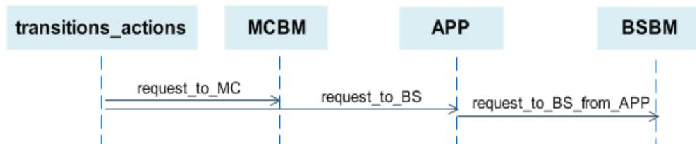
Figure 4.8: Signals generated by the *transitions\_actions* process
