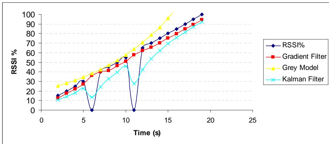
Figure 3.8: Filters results on synthetic RSSI values of shape B
