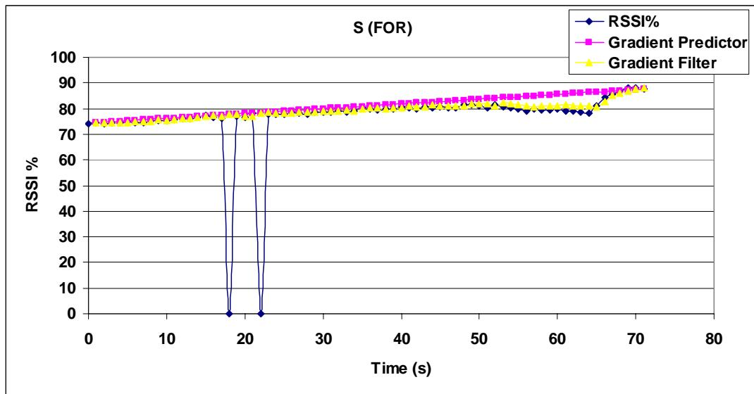
Figure 3.24: Gradient Filter test on RSSI measured values in the direction S (FOR)
