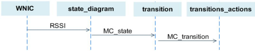
Figure 4.4: Signal exchange to generate MC state and transition
