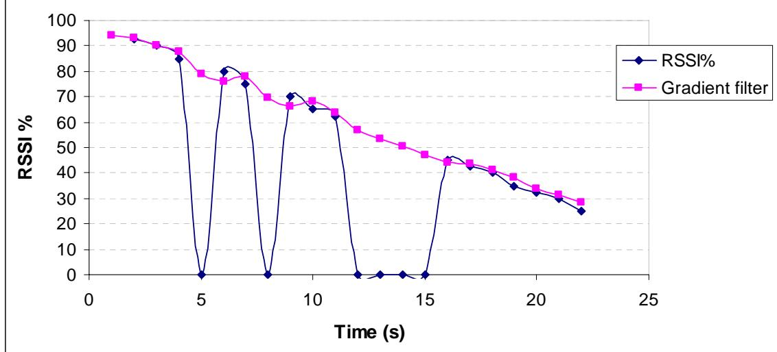
Figure 3.14: Gradient Filter output in the presence of continuous zeros
