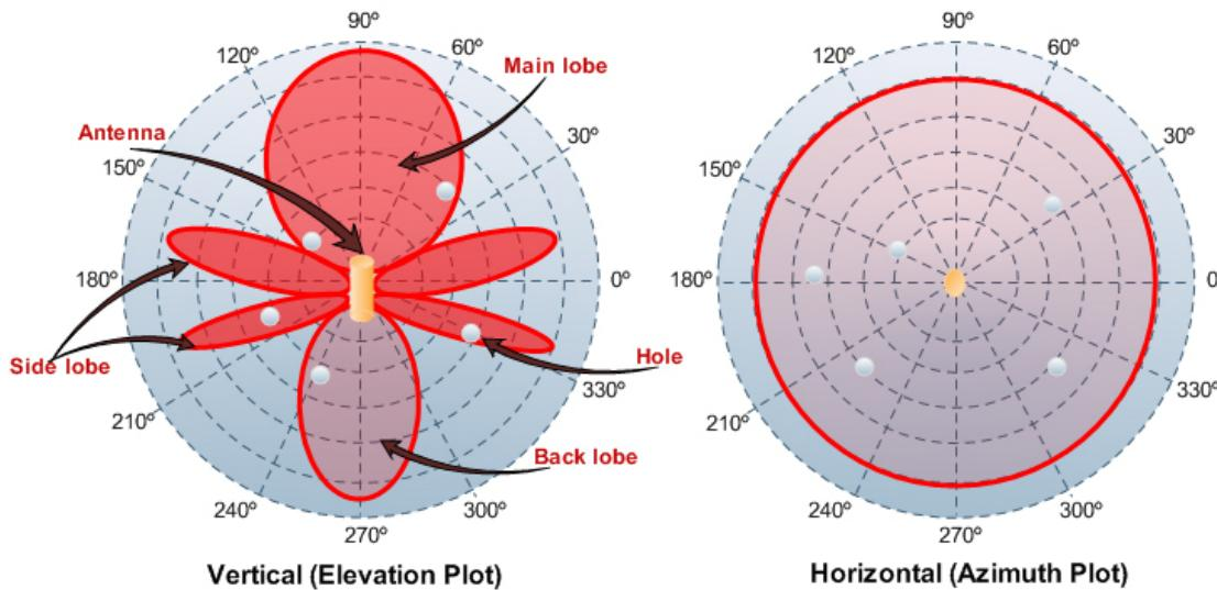
**Figure 1.3: Real CA (antenna radiation)**
