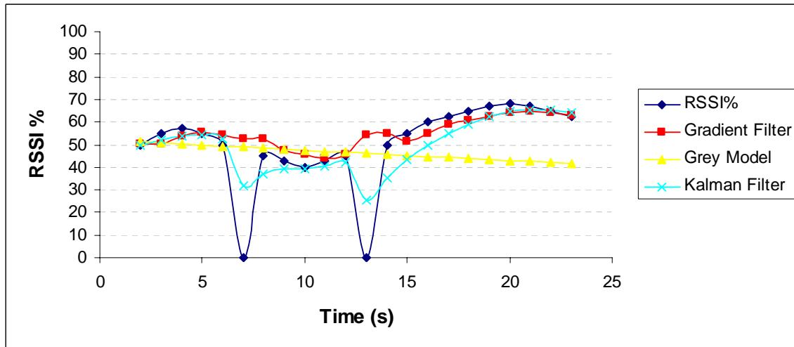
Figure 3.12: Filters results on synthetic RSSI values of shape F
