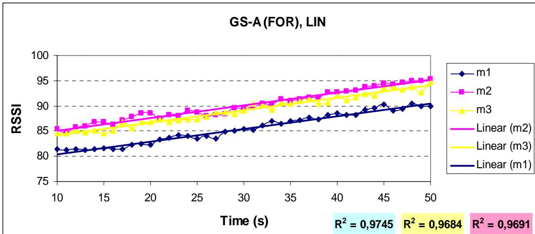
Figure 3.18: Linear trendline of RSSI% in the direction GS-A (FOR)
