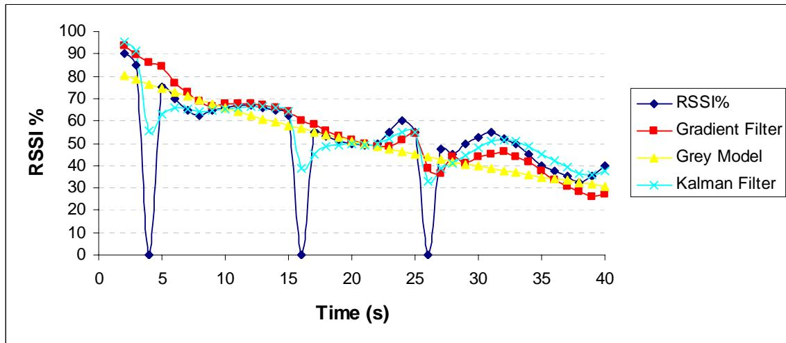
Figure 3.13: Filters results on synthetic RSSI values of shape G
