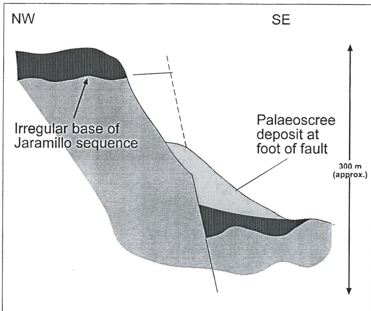
Fig. 20.- Schematic cross-section showing estimated offset across the San Andrés fault, south of the Barranco de Tiñor.
