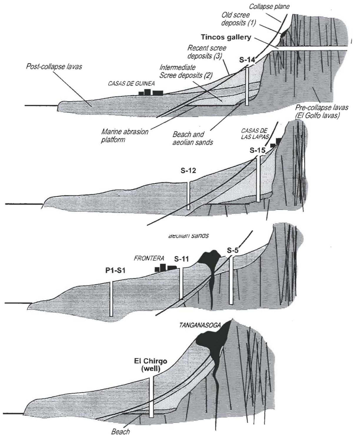
Fig. 15.- Different cross sections inside the El Golfo embayment based on information from the boreholes.
