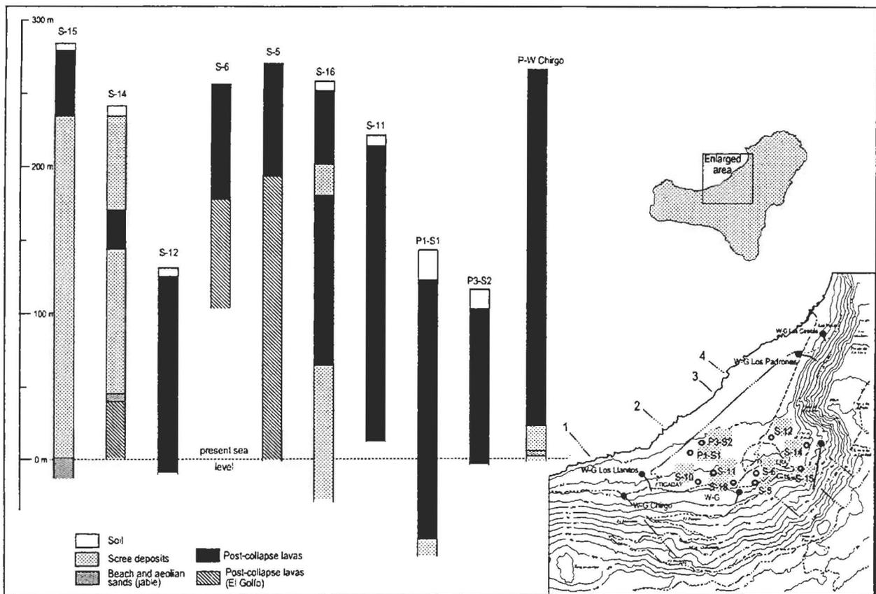
Fig. 14.- Geological columns of boreholes drilled for underground water exploration inside the El Golfo embayment.
