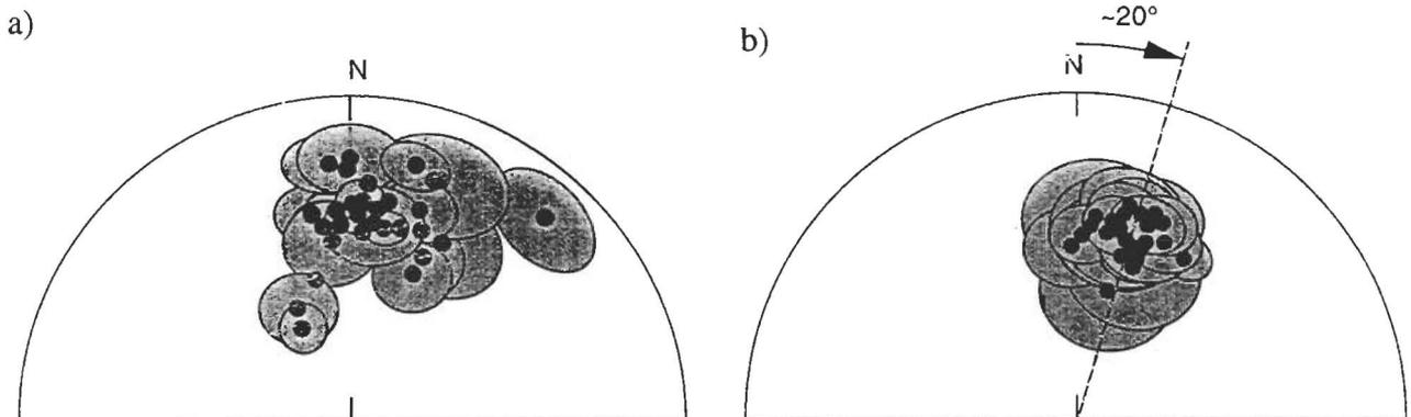
Fig. 24 .- Declination, inclination and VPG latitudes and longitudes obtained from volcanics of the El Golfo section (Ermita de La Peña). Stereographic projections of the palaeomagnetic directions obtained for the upper part (a) and lower part (b) of the El Golfo section show a 20° rotation affecting the lower El Golfo.
