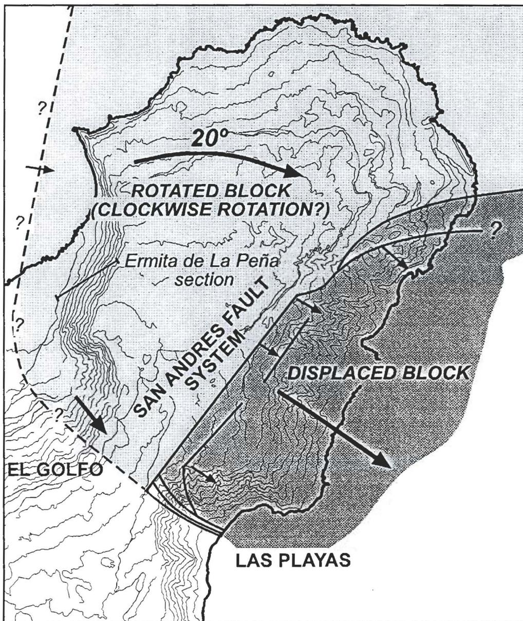
Fig. 25.- An interpretation of the rotation of the lower El Golfo evidenced by palaeomagnetism: This rotation would be associated with the San Andrés fault, as a main lateral collapse during the development of the lower part of El Golfo volcano.
