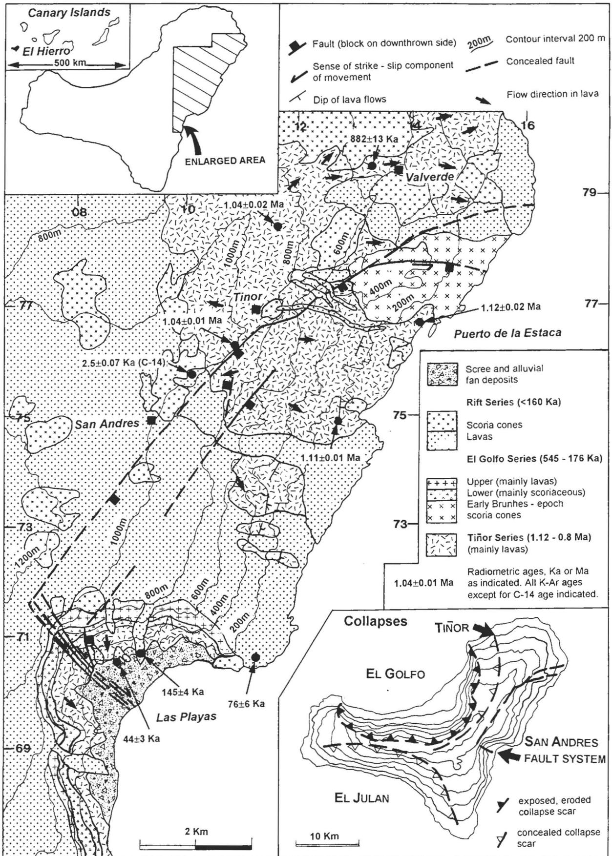
Fig. 19.- Geological map of eastern El Hierro, showing relationships of lithostratigraphic units to the San Andrés fault system. Insets show location of El Hierro and positions of other collapse structures on the island.
