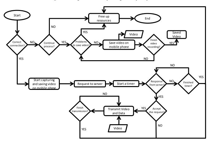
Figure 10. Algorithm for improving the request process.
