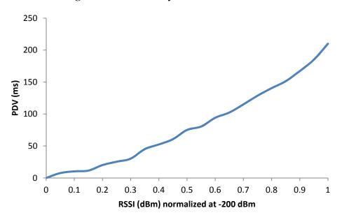
Figure 14. Packet delay variation versus RSSI.
