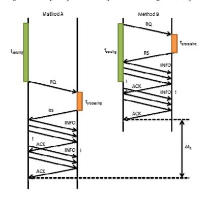
**Figure 8.** Request process comparison with higher t<sub>sensing</sub>.
