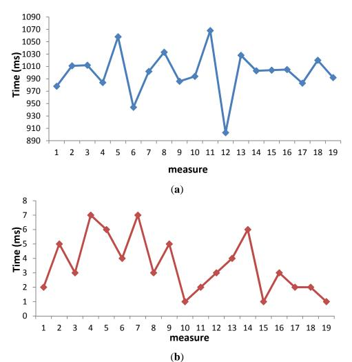
**Figure 12.** Time needed to read the values of the sensors ( $T_{sen}$ ).
