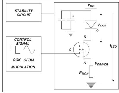
Fig. 1. Model of a LED modulating circuit.
