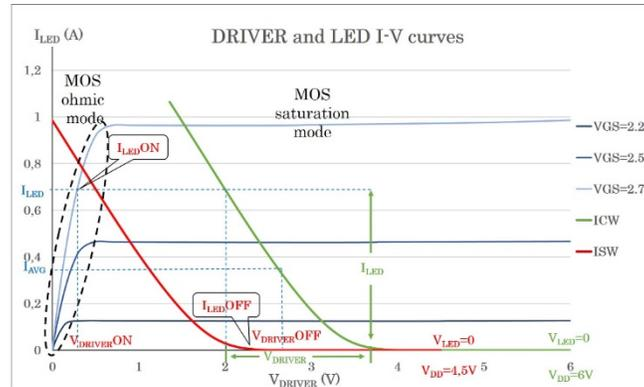
Fig. 2. I-V joint curves for the MOS (blue) and LED (red and green). The vertical axis represents the current  $I_{LED} = I_{DRIVER}$ . The horizontal axis represents the MOS voltage ( $V_{DRIVER}$ ) starting at the origin ( $V_{DRIVER} = 0V$ ). Starting at  $V_{DRIVER} = 6V$  and going backwards, the horizontal axis represents the LED voltage ( $V_{LED}$ ). Notice that  $V_{DD} = V_{DRIVER} + V_{LED}$ .
