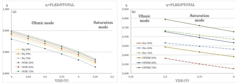
Fig. 3. Summary of results for the energy efficiency ratio  $\eta$ . (a) ohmic mode (switched and OOK signals) and (b) saturation mode (sinusoidal and OFDM signals). It can be seen how  $\eta$  drops when increasing the power supply  $V_{DD}$ . Furthermore, the CW signals energy efficiency ratio radically decreases for low illumination values.
