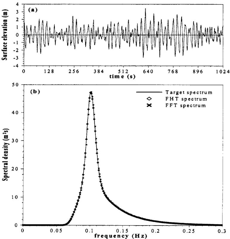
Figure 1: Simulated wave record (a), target spectrum and spectral density function estimated via FHT and FFT (b).
