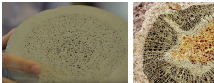
Figure 2 : Varied densification FGAM concrete by Keating mimicking the radial density gradient of a palm tree [5].
