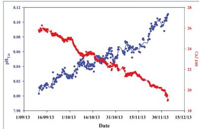
Saronikos buoy record of pH in total scale at in-situ conditions of temperature and salinity (blue dots) and sea surface temperature (SST in °C, red dots) from deployment day September 10 to December 5, 2013.
