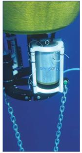
(Left) Immersed part of the VULCANO buoy with the SensorLab pH sensor. (Bottom) VULCANO buoy record of pH in total scale at in-situ conditions of temperature and salinity (blue dots) and sea surface temperature (SST in °C, red dots) from deployment day November 7 to December 8, 2013. (Right) Saronikos buoy with pH sensor before deployment in September 2013.
