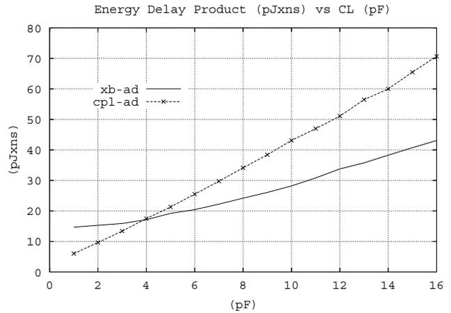
Figure 6. Energy-delay product versus loading for STM 65nm process.
