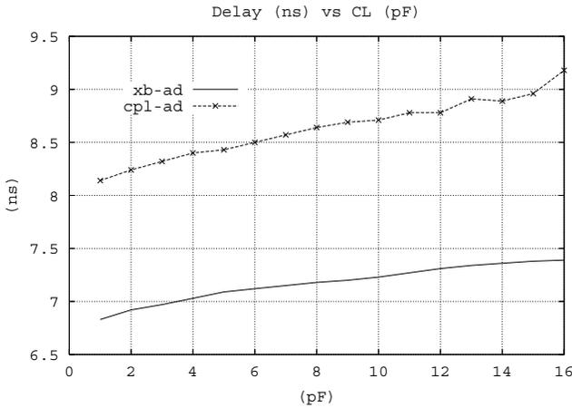
Figure 4. Propagation delay time versus output load capacitance for STM 65nm process.
