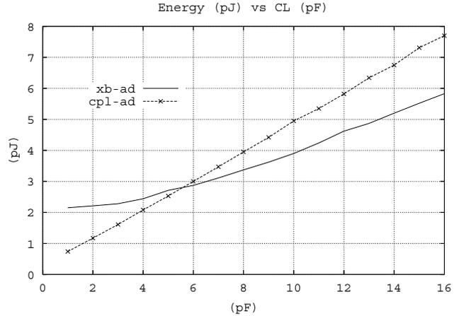
Figure 5. Energy versus loading for STM 65nm process.
