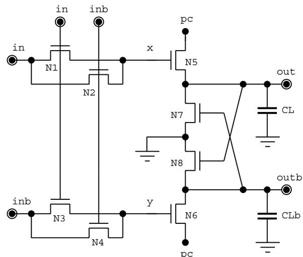
Figure 1. Circuit structure of *cpl-ad*.
