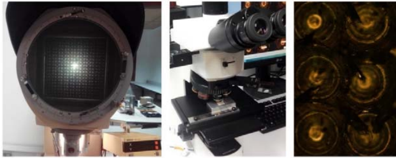
Fig. 4. Measurement equipment used in geometric characterization and micro burrs.
