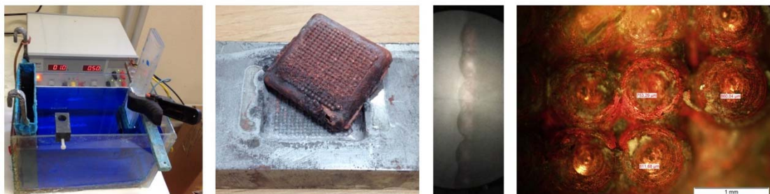
Fig. 6. Electroforming equipment, copper shell obtained, side profile view and microscope image with measurements.
