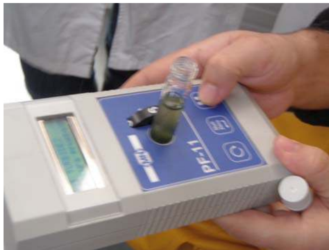
Figure 23. Macherey-Nagel compact photometer pf-11 used to calculate the water turbidity due to cell concentration.
