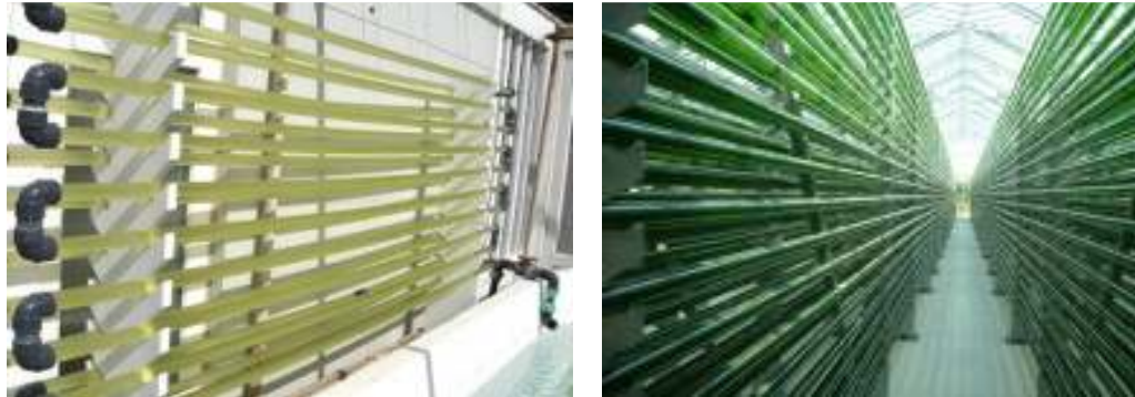
Figure 9. Left. Horizontal tubular photo-bioreactor in ICCM fish hatchery. Right. Industrial tubular photo-bioreactor for biofuel production. http://brae.calpoly.edu/CEAE/images/biofuels3.gif
