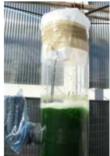
Figure 67. A) VPbrs settled outside the mesocosmo facilities at ICCM's Hatchery. B) VPbr I equipped with a water pump and air supply. C) VPbr II equipped just with air supply and continuous \text{CO}_2 gas income.
