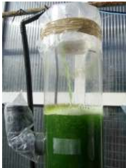
Figure 67. A) VPbrs settled outside the mesocosmo facilities at ICCM's Hatchery. B) VPbr I equipped with a water pump and air supply. C) VPbr II equipped just with air supply and continuous \text{CO}_2 gas income.
