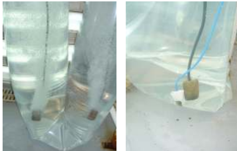
Figure 12. Left, one air diffuser on each side of the bag. Right, just one CO 2 diffuser (blue hose) per bag.
