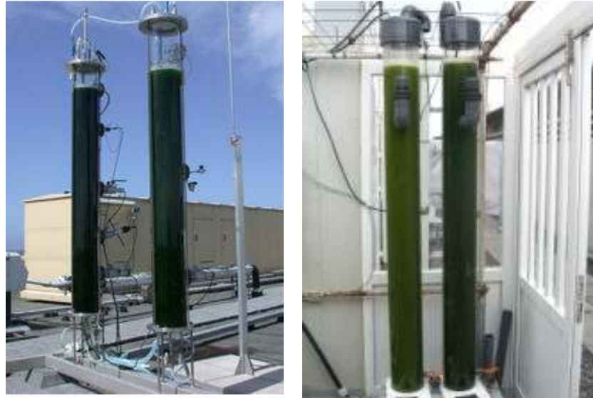
Figure 8. Vertical column photo-bioreactors. Left. http://www.bioenergy-noe.com Right. ICCM's fish hatchery vertical photo-bioreactors.
