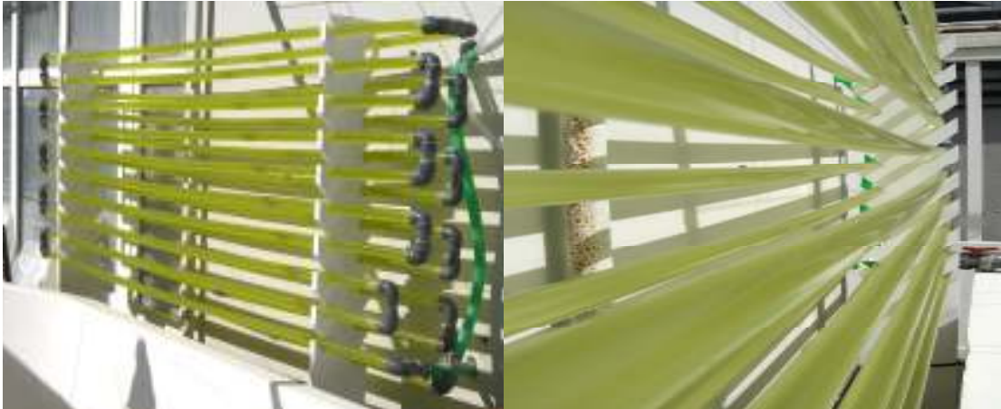
Figure 91. The outdoor methacrylate tubular structure of the HPbr.
