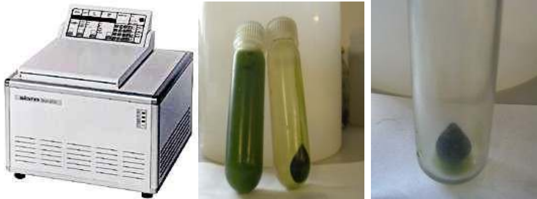
Figure 27. A. Sigma centrifuge used to separate algae cells from water. B. Algae sample flasks before and after centrifugation. C. Algae pellet after removing supernatant
