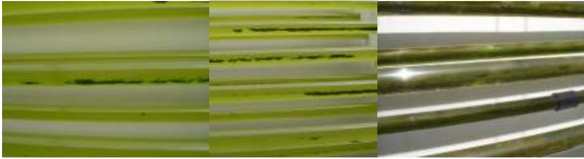
Figure 93. Cell deposition and diatoms attached inside the methacrylate tubes. A) at the 15 th culture day, B) at the 22 nd culture day and C) At the lasts days of the experiment.
