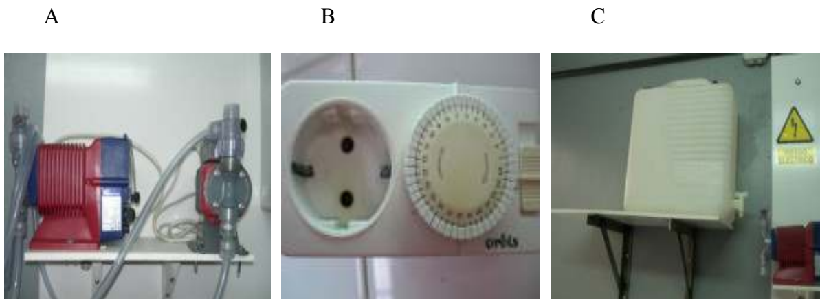
Figure 15. A: Iwaki™ peristaltic pump to add enriched water during sunlight hours. B; Orbis timer commanding the peristaltic pump to work during daylight hours. C; plastic container with enriched water.
