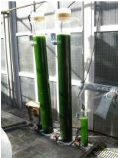
Figure 67. A) VPbrs settled outside the mesocosmo facilities at ICCM's Hatchery. B) VPbr I equipped with a water pump and air supply. C) VPbr II equipped just with air supply and continuous \text{CO}_2 gas income.
