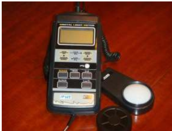
Figure 25. Digital light meter HT 170N used for Light irradiance measures.
