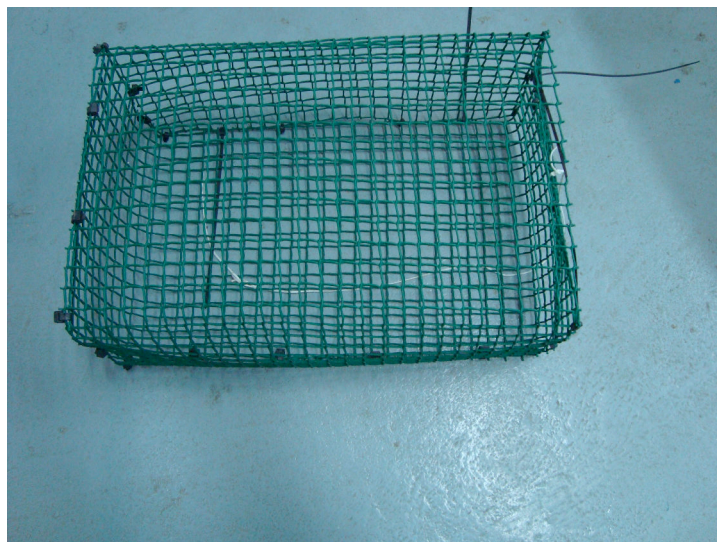
Figure 2.5: A sample of cage used for stress panel tests.
