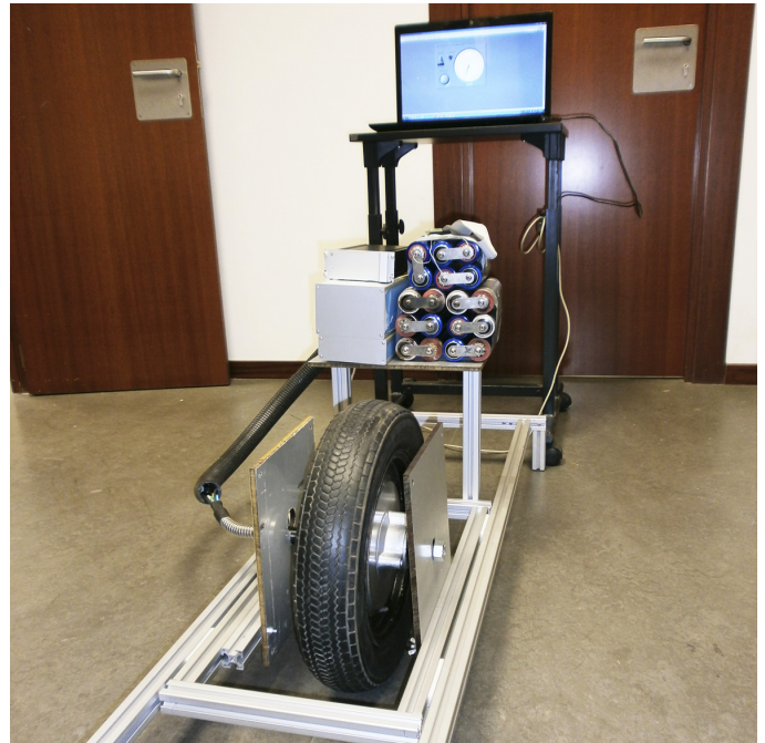
Fig. 10. View of the test bench of BLDCM control system for electric vehicles
