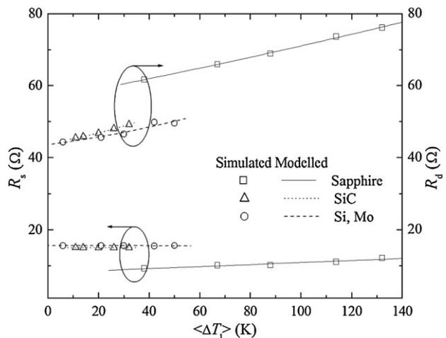
**Figure 4**  $R_{\text{S}}$  (left axis) and  $R_{\text{D}}$  (right axis) against average channel temperature increment for sapphire, SiC and Si or Mo substrates (Si and Mo data are fully overlapped). Numerical data are represented with squares, triangles and circles, and modelled data with solid, dotted and dashed lines, respectively.
