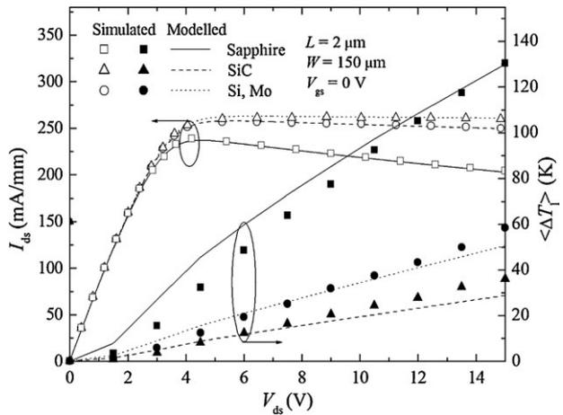
**Figure 5** Output characteristics (left axis) and  $\langle \Delta T_1 \rangle$  (right axis) vs. drain voltage for sapphire, SiC and Si or Mo substrates (Si and Mo data are fully overlapped). Numerical data are represented with squares, triangles and circles, and modelled data with solid, dotted and dashed lines, respectively;  $V_{gs} = 0 \text{ V}$ .
