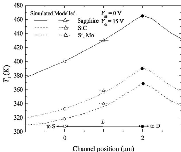
**Figure 6** Simulated local channel temperature vs. channel position along the longitudinal direction, for the different substrates, is shown in lines. Circles represent the location of the borders of the gate, being solid at the drain side of the gate. The average channel temperature obtained with the model, accounting for SHEs, is shown by hollow triangles (a horizontal line has been added in this case to ease the comparison with the local temperature);  $V_{gs} = 0$  V and  $V_{ds} = 15$  V.
