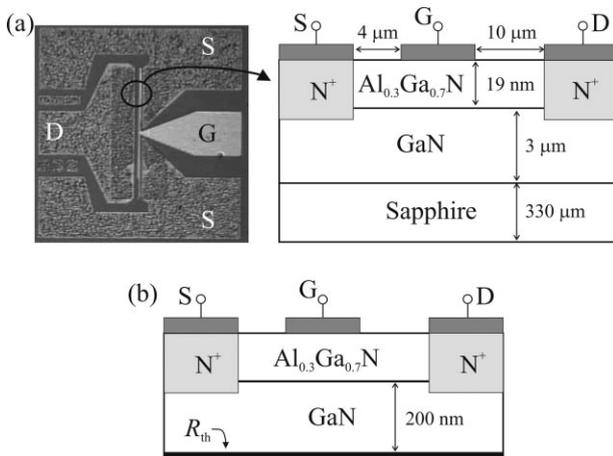
**Figure 1** (a) AlGaN/GaN on sapphire HEMTs structure (not to scale). (b) Equivalent thermal resistance,  $R_{\text{th}}$ , at the bottom of the structure.
