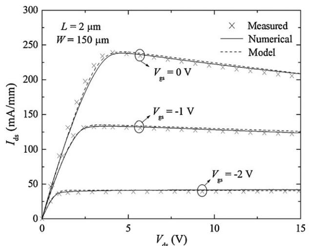
**Figure 3** Sapphire HEMTs output characteristics. Measured, simulated and modelled data are represented with crosses, solid lines and dashed lines, respectively;  $V_{\text{gs}} = -2, -1$  and 0 V.
