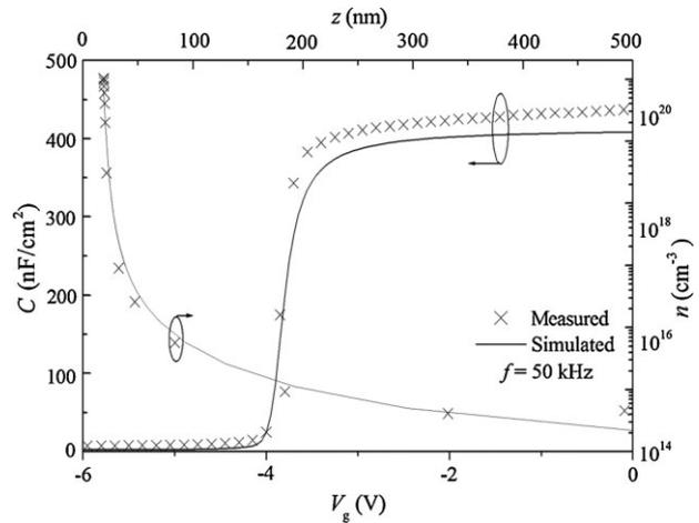
**Figure 2**  $C$ - $V$  characteristics (left axis) and electron profile against the depth from the AlGaN top surface (right axis). Measured and simulated data are represented with crosses and solid lines, respectively.
