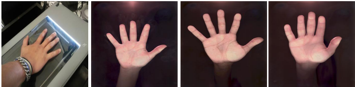
Figure 4. Scanner acquisition (figure on the left) and acquired hand images from three different users (three figures on the right).
