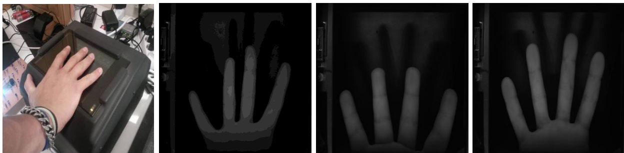
Figure 5. PRM acquisition device (figure on the left) and acquired IR hand images from three different users (three figures on the right).
